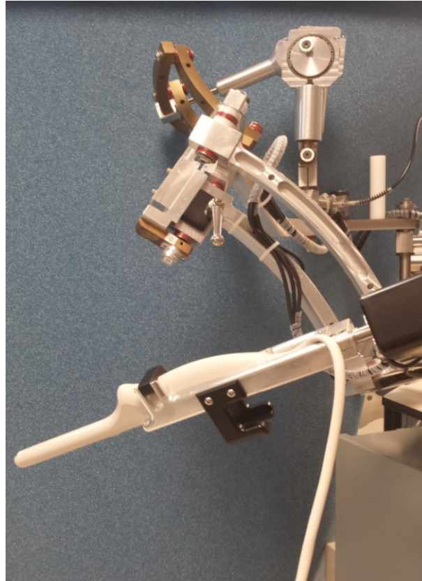
Figure 1.8: A photograph of the mechanically-assisted 3D TRUS biopsy system with real-time tracking and recording of the 3D position of biopsy needle.
